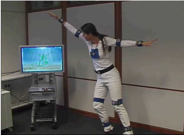
Figure 1: Dancer wearing wireless motion capture sensors
